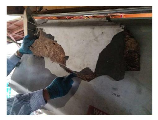
The above photo shows the item matched the Right-Hand Nose Gear Forward Door. The photo below shows the oval depressions and the raised diagonal bar.
