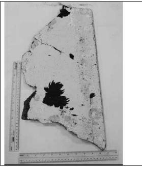
After review of the B777 Illustrated Parts Catalogue (IPC), the most possible location of the part was determined to be the wing to fuselage body fairing. The location of where the part was
